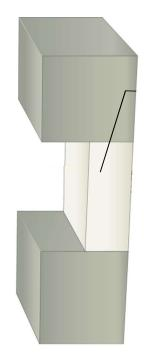
Protecta EX Mortar Minimum seal depth 100mm Maximum aperture 1200x2400mm
